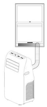
**NOTE**: The length of the exhaust duct is variable between 480 mm and 1500 mm (adaptors included). Using a shorter length of ducting uses less energy.
