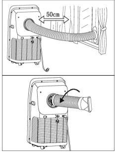
5. Move the air conditioner into position and extend the flexible exhaust duct to suit your window layout.
